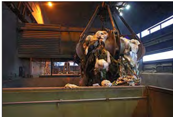
At Covanta Energy's waste-to-energy facility in Alexandria, Va., a claw drops trash into a combustion chamber, which will burn the waste at about 2,000 degrees Fahrenheit. Photo by Emily Yehle.
